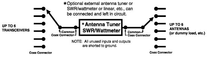
CONNECT ANY TRANSCEIVER TO ANY ANTENNA.
